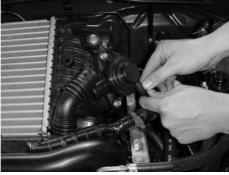
2) Remove the securing bolts and remove the standard BOV
