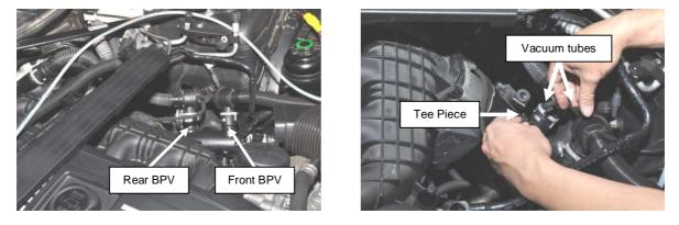
9) Remove the 2 standard bypass valves (BPV's) and their plumb back hoses by rotating the grey securing clips clockwise and pulling them out.
