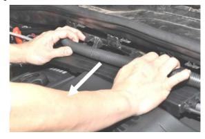
5) Remove the securing bolts holding the shroud in and remove the shroud.
