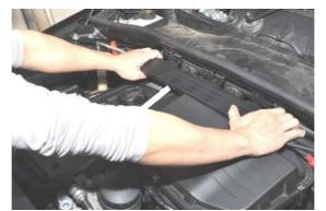
4) Unclip the 3 clips on the shroud and remove the wiring.
