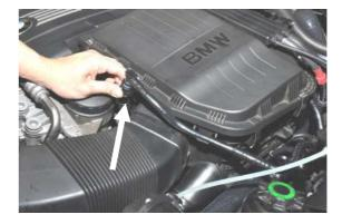
7) Unclip the intake snorkel and remove air box by pulling it up off its rubber mounts
