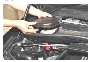
3) Pull the wiring harness cover towards the front of the car to slide it off the clips on the shroud
