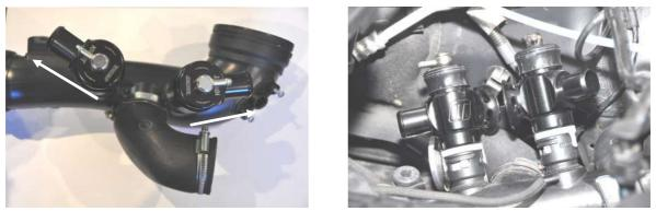
13) Install the recirculation hoses. Secure hoses with supplied hose clamps.
