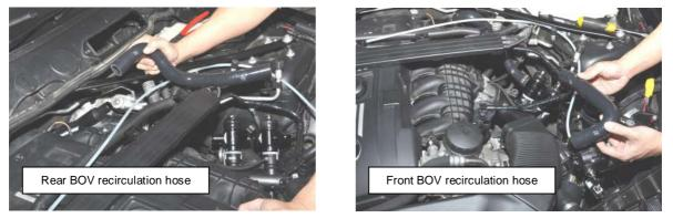
14) Connect the supplied vacuum tube to the tee piece and the Kompact BOV's. Use the 3mm spring clamps to secure the vacuum tube onto the standard tee piece and the 5mm spring clamps to secure the hose to the BOV nipples.
