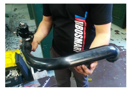
5. Reinstall the hot-pipe onto the compressor cover. Use the supplied hose reducer and hose to connect the OEM hose to the Turbosmart BOV. Ensure that all hose clamps and spring clamps are installed. The 6mm hose clamp is used for securing the OEM vacuum hose onto the reducer fitting. One 5mm hose clamp is used to secure the supplied 5mm vacuum hose onto the reducer fitting, the other is to secure the vacuum hose to the BOV nipple.
