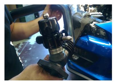
4. Before reinstalling the hot-pipe, ensure that the clamp is tightened and that the BOV orientation is same as OEM.
