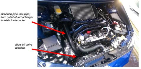
2. Loosen the clamp that is securing the BOV onto the hot-pipe. Gently pull the OEM BOV away from the hot-pipe to remove it.
