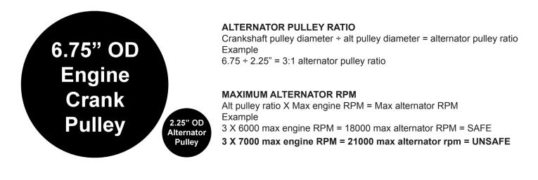
If your max calculation is greater than 18000 alternator RPM's, increase the alternator pulley diameter or decrease the crank pulley diameter to compensate. If changing the alternator pulley is not possible, use an engine rev limiter to control maximum engine RPM's.
