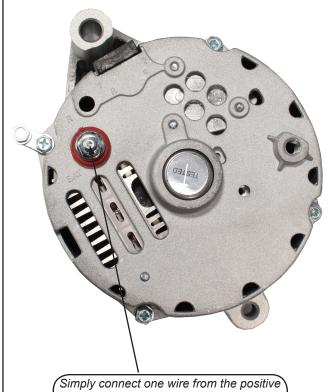
Simply connect one wire from the positive battery terminal to the positive alternator terminal. It's that easy!
