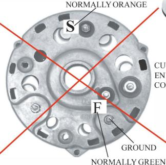
CUT THE EYELETS OFF THE ORIGINAL HARNESS WIRE ENDS FROM "S" & "F" TERMINALS. CRIMP ON NEW CONNECTORS PROVIDED
