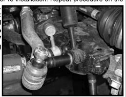
12. Working on the driver side, remove the sway bar end link hardware that connects the sway bar end link to the lower control arm. Save the hardware for later re-installation. Repeat procedure on the passenger side. Let the stock sway bar hang.
