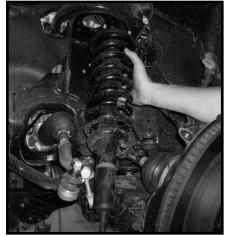
14. Working on the driver side strut, measure the exposed threads sticking out of the middle bolt on the strut.
