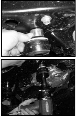
33. Locate the skid plate and the skid plate hardware. Install the skid plate into the OE location and secure using the hardware. Make sure to use loctite and torque all skid plate mounting hardware to **18 ft lbs.**
