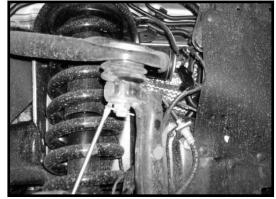
6. Working on the driver side, loosen but do not remove the nut that connects the upper control arm ball joint to the steering knuckle. Carefully break the taper by striking the knuckle with a hammer. Special note: Take special care not to damage the upper control arm ball joint or rip the upper control arm ball joint dust boot. For now, leave the upper control arm attached to the knuckle. We want to just break the taper for now. Repeat procedure on the passenger side.
