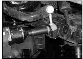
13. Carefully lower down on the hydraulic floor jack about 2" allowing enough room for the strut to be removed from the vehicle. Repeat procedure on the passenger side.
