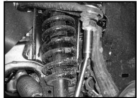
7. Working on the driver side, remove the cotter pin from the outer tie rod ball joint. Save the cotter pin for later reinstallation. Repeat procedure on the passenger side.
