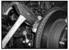
9. Move back to the upper control arm ball joint nut and remove completely. Also, move back the outer tie rod ball joint nut and remove completely. Remove the upper control arm and the outer tie rod from the knuckle. Let the knuckle hang. Special note: Make sure not to over extend the brake lines, ABS lines and the CV axle, if need be, tie the knuckle up so these problems do not happen. Repeat procedure on the passenger side.
