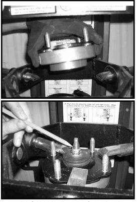
18. Locate (4) S10090 sleeves from hardware bag 52070NB. Locate the (4) upper OE nuts. Also, locate the newly modified strut. Working on the driver side, install the modiffied strut into the upper location and secure using the OE nuts. **Do not tighten at this point.Special note: Make sure that the out arrow is facing towards the outside of the vehicle.**
