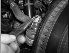
27. Locate the brake line mounting hardware. Working on the driver side, secure the brake line bracket to the knuckle and secure using the OE hardware. Make sure to add some loctite and torgue to **12 lbs.**
