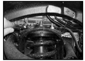
5. Working on the driver side, remove the cotter pin from the upper control arm ball joint. Save the cotter pin for later re-installation. Repeat procedure on the passenger side.
