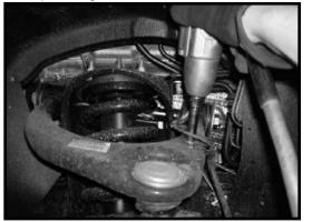
3. Working on the driver side, remove the hardware that connects the brake line bracket to the knuckle. Save the hardware for
