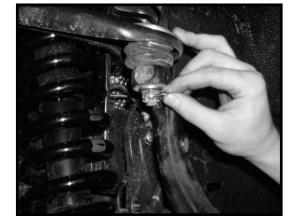
19. Locate the sway bar end link mounting hardware. 25. Locate the outer tie rod castle nut. Working on the driver Working on the driver side, secure the sway bar end link to side, install the outer tie rod the knuckle and secure using the lower control arm using the OE hardware. Add some loc-tite and torque to **60 ft lbs**.
