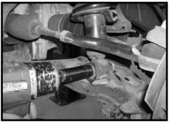
4. Working on the driver side, loosen but do not remove the stock nut that connects the stock upper control arm to the stock knuckle. Carefully break the stock taper of the upper control arm ball joint then remove the stock nut completely and set aside. Separate the stock upper control arm and
