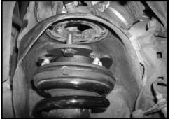
9. Locate the stock lower strut hardware. Working on the driver side, install the modified stock strut into the stock lower control arm location using the stock hardware. Make sure to use thread locker or loctite and torque to **155 ft lbs.** Repeat procedure on the passenger side.
