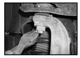
stock nut connecting the stock upper ball joint to the stock knuckle. Repeat procedure on the passenger side.
