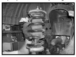
11. Locate the new strut spacers and the stock hardware Working on the driver side strut, <u>install the new spacer</u> on top of the stock strut and secure using the stock hardware. Make sure to use thread locker or loctite and torque to **48 ft lbs**. Repeat procedure on the passenger side strut.
