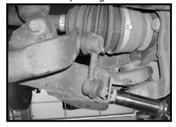
Locate the stock upper control arm mounting hardware. Working on the driver side, attach the stock upper control arm to the stock knuckle and secure using the stock nut. Tuff Country EZ-Ride Suspension packages some post upper control arm down so that it can be attached to the stock knuckle. Repeat procedure on the passenger side.
