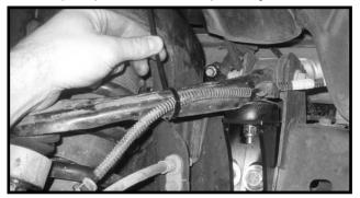
15. Remove the hydraulic floor jacks from under the lower control arms and check and double check to make sure all steps were performed properly.
