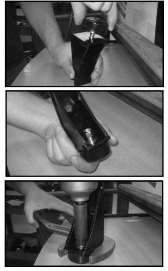
13. Locate (2) 32102-03 specialty washers, (2) 1/2" x 4" bolts, (4) 7/16" USS flat washers and (2) 1/2" unitorque nuts from hardware bag 32103NB. Working on the driver side, install the bump stop bracket to the frame rail under the rear portion of the upper control arm (hole provided) and secure using the new hardware. Special note, the specialty wash-
