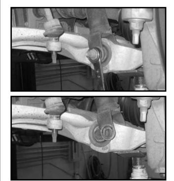
5. Working on the driver side, place a reference mark on the cam washer and cam stops that attach the lower control arm to the front and rear lower control arm mounts. Repeat procedure on the passenger side.
