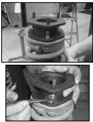
9. Locate (6) 3/8 nylon nuts and (6) 5/16" USS flat washers from hardware bag D2P-NB. Working on the driver side, install the newly modified coil over into the upper location and secure using the new hardware. Make sure to use loc-tite and torque to **32 ft lbs.** Repeat procedure on the passenger side.
