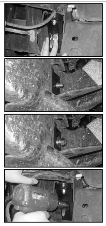
14. Locate the (2) zip ties in hardware bag 32103NB. Working on the driver side, zip tie the ABS line to the upper control arm so that ABS line does not get pinched between the upper control arm and the newly installed bump stop bracket. Repeat procedure on the passenger side.
