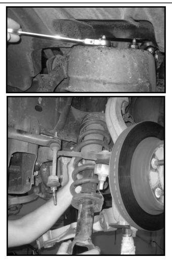
Install the new front spacers on the coil overs using the OE hardware. Make sure to use loctite and torque to 32 ft lbs.
