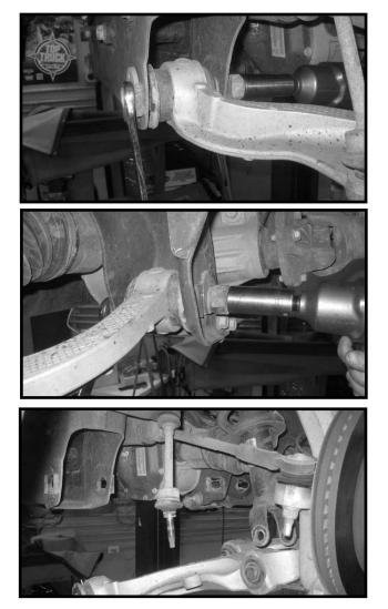
7. Working on the driver side, remove the (3) nuts that attach the coil over into the upper location. Save the hardware. Remove and set the coil over aside. Repeat procedure on the passenger side.
