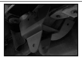
4. Working on the driver side and using the newly installed front traction bar bracket as a guide, carefully drill 3 holes into the OE hanger. Repeat procedure on the passenger side.
