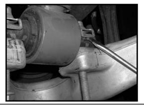
11. Locate the upper control arm mounting hardware. Place a hydraulic floor jack under the driver side lower control arm and carefully raise up on the hydraulic floor jack until the upper control arm can be attached to the knuckle. Secure using the hardware and torque to **65 ft lbs.** Repeat procedure on the passenger side.
