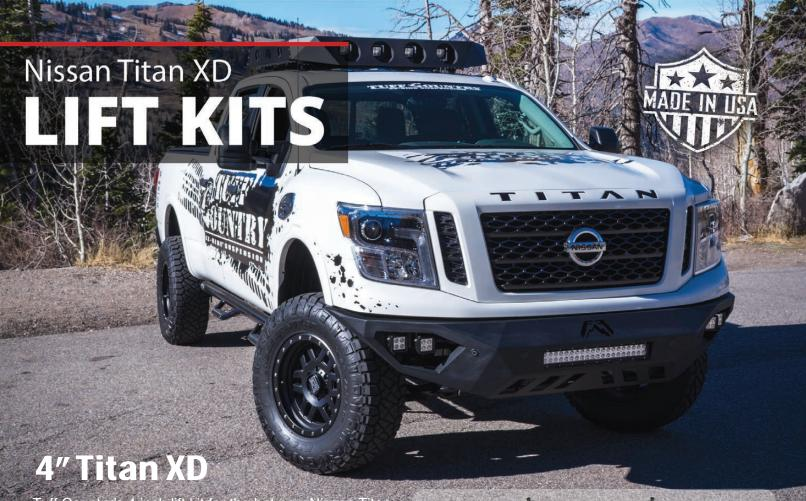
Tuff Country's 4 inch lift kit for the hot new Nissan Titan XD will allow for up to 33" tires (35" with trimming). Installs easily using a combination of upper control arms and coil/strut spacers to lift the front end. Rear 2" lift blocks raise the rear end.
