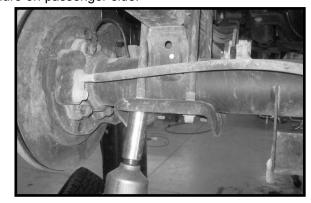
44. Working right above the rear drive line, remove the OE emergency brake line brackets from the OE location. Save the hardware.
