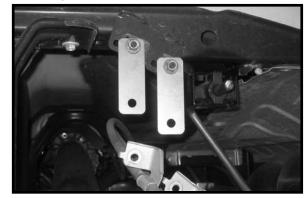
46. Locate (2) 5/16" x 1" bolts, (4) 1/4" USS flat washers and (2) 5/16" unitorque nuts from hardware bag 54060NB. Secure the OE emergency brake line brackets to the newly installed emergency brake line brackets and secure using the new 5/16" hardware. Make sure to use loctite and torque to **22 ft lbs.**
