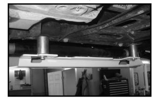
Carefully remove the (2) hydraulic floor jacks from under the lower control arm.
