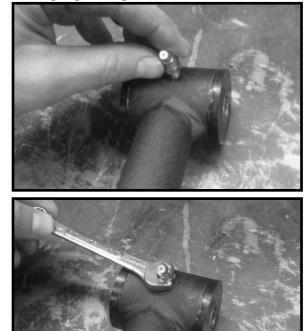
26. Working on the driver side, install the new upper control
