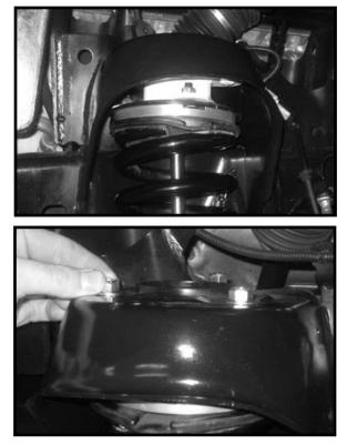
22. Working on the driver side, secure the bottom portion of the strut to the lower control arm using the OE hardware. Make sure to use loctite and torque to 150 ft lbs. Repeat procedure on the passenger side.
