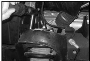
12. Working on the driver side, remove the lower mounting hardware that attaches the strut to the lower control arm. Save the hardware. Carefully lower down on the hydraulic floor jack allowing removal of the strut easier. Remove the strut and set aside. Repeat procedure on the passenger side.
