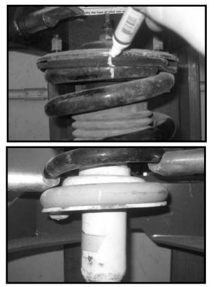
14. Place a clamp on the bottom coil portion of the coil spring and strut plate. This will help keep the coil spring in the proper location.
