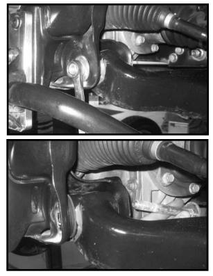
31. Locate (4) 9/16" x 5" cam bolts and (8) cam washers from hardware 54060NB1. Also, locate (4) 9/16" unitorque nuts from hardware bag 54060NB. Working on the driver side, secure the lower control arm to the OE mounting points using the new cam bolt and hardware. Make sure to use loctite and torque to **100 ft. lbs.** Repeat procedure on the passenger side.
