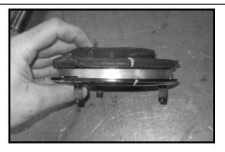
18. Working on the driver side strut, install the bearing plate, pre load spacer and isolator back to the strut and securing using the OE hardware. Make sure to us loctite. **Special note: Make sure that the lines that were scribed earlier in the installation line up with each other.**
