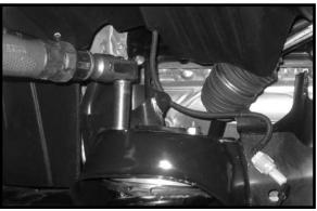
24. Locate the new upper control arms. Locate (8) poly arm into the upper pockets using the OE hardware. Do not bushings and (4) S10243 sleeves from hardware bag tighten at this point. Repeat procedure on the passenger 54060PL. Install the new bushings and sleeves into the new side.
