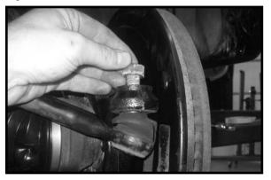
29. Working on the driver side, secure the brake line bracket back to the brake line location using the OE hardware. Make sure to use loctite and torque to **8 ft lbs.**
