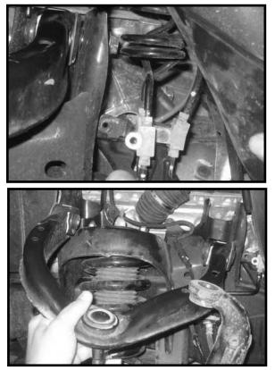
10. Working on the driver side, carefully remove the hardware attaching the outer tie rod to the knuckle. Save the hardware. Carefully break the taper and remove the tie rod from the knuckle. **Special note: Take special care not to damage the ball joint boot during removal.** Repeat procedure on the passenger side.
