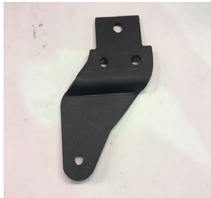
Part # 54050-05 Passenger side rear sway bar bracket
