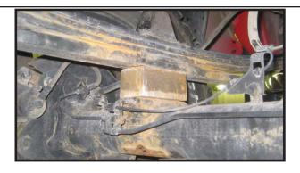
26. Locate (4) 9/16" x 2 9/16" x 9 5/8" square u-bolts. Locate (8) 9/16" u-bolt high nuts and (8) u-bolt washers from hardware bag 916NW. Also, locate the lower u-bolt plates. Working on the driver side, install the new u-bolts into the stock location and secure using the new 9/16" high nuts and washers. **Special note: If need be, cut off the excess threads off each leg of the newly installed u-bolts.** Torque to **120 ft lbs.** Repeat procedure on passenger side.
