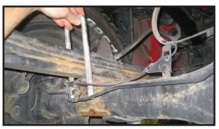
24. Carefully lower down on both hydraulic floor jacks at the same time allowing enough room for the rear blocks to be installed. **Special note: Take special care not to over extend any brake lines and/or hoses.**
