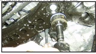
OE mount and secure using the new 1/2" hardware, make sure to use the OE over size washer on the head side of the 2. Remove the skid plate from the OE location. Save the bolt. Repeat procedure on the passenger side. Move back to the new hardware hardware on the driver and passenger side and add some loctite and torgue to 55 ft lbs.
