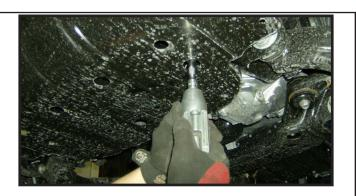
3. Working on the driver side, remove the hardware that At the end of the installation take the same measure-attaches the front portion of the differential to the OE ments and compare to the pre-installation measure-mounts. Save the over size washer on the head side of the bolt. Repeat procedure on the passenger side
