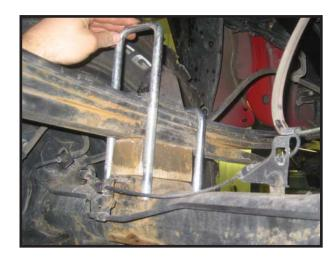
27. Reinstall the lower shock mounting locations using the OE hardware.
