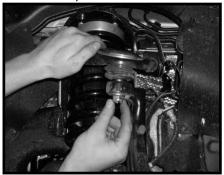
nut does not line up with the stock ball joint, DO NOT 12 lbs. loosen the stock castle nut so that the cotter pin can fit, tighten the stock castle nut some more so that the stock cotter pin can be installed.
