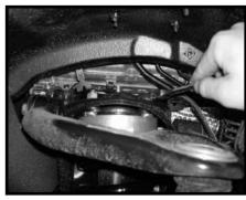
19. Locate the stock sway bar end link mounting hardware. Working on the driver side, secure the stock sway bar end link to the stock lower control arm using the stock hardware. Add some thread locker or loctite and torque to **60 ft lbs.**
