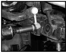
13. Carefully lower down on the hydraulic floor jack about 2" allowing enough room for the stock strut to be removed from the vehicle. Repeat procedure on the passenger side.
