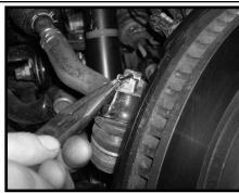
27. Locate the stock brake line mounting hardware. Working using the stock castle nut. Make sure to add some thread sure to add some thread locker or loctite and torque to 12 lbs.
