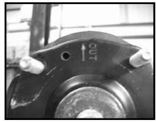
18. Locate (4) S10090 sleeves from hardware bag 53070NB. Locate the (4) stock upper strut nuts. Also, locate the newly modified stock strut. Working on the driver side, install the modified stock strut into the stock upper location and secure using the stock nuts. **Do not tighten at this point. Special note: Make sure that the out arrow is facing towards the outside of the vehicle.**
