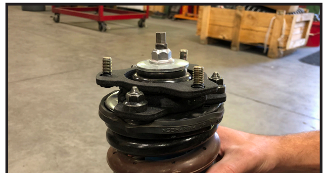
17. Locate part # 52915-01 and the three OE upper strut nuts. And install on to the strut. Tighten to 36 ft-lb . Special note. If OE strut studs are higher than the new spacer. Grind off the tip of the studs.
