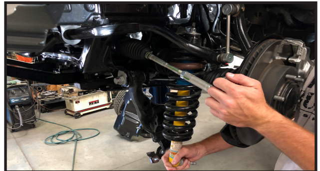
17. Locate part # 52915-01 and the three OE upper strut nuts. And install on to the strut. Tighten to 36 ft-lb . Special note. If OE strut studs are higher than the new spacer. Grind off the tip of the studs.
