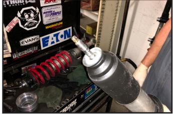
Re-install the shock absorber into the strut assembly an make sure to line up your reference marks made on step #8.
