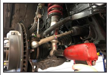
trol arm ball joint piece to the steering knuckle.
