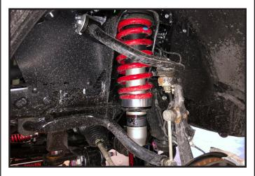
16. Raise the lower control arm back up until you can install the OE lower mounting bolt and hardware. Leave this loose for now.
