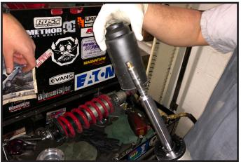
11. Locate a new strut spacer part # 51020-01 and install it over the body of the shock. Make sure to install the new spacer so that the "coil shelf" is facing upwards.
