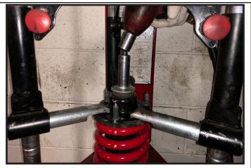
10. Remove the shock absorber from the strut assembly out of the bottom of the coil spring. Remove the metal washer and plastic dust boot. Save for re-installation
