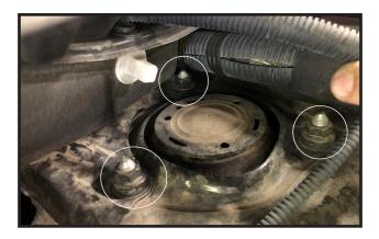
3. Locate the new strut spacer plates and install 1 each on top of the OE struts over the 3 studs.
