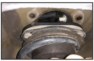
4. Once the new spacers have been installed, carefully raise both sides of the front suspension so that the upper strut studs go back through the original holes of the vehicle. 5. Locate the new 10mm star washers and 10mm fine nuts. Install the star washer first, then the nut, Torque to **30ft lbs**.
