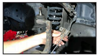
7. Remove the rubber grease boot from the upper ball joints,
