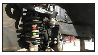
19. Move back to the 9/16" x 5" bolts and tighten to **125 ft Ibs.**
