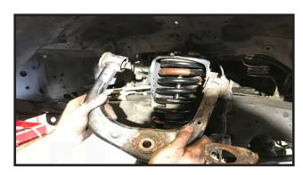
13. Locate the new upper control arms, driver side is part # 50965-01 and passenger side is 50965-02. Also locate (8) poly bushings, (4) S10254 crush sleeves, and (4) SERT06 grease fittings from hardware bag 50965NB1. Carefully install the grease fittings into each eyelet of the new control arms. Take extra care to not over tighten these as they are small brass fittings. Make sure they are facing towards the outside of the vehicle for proper greasing access.
