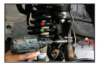
21. Locate and install the 3/8" x 1" bolts into the center threaded hole of the knuckle support brackets. This bolt is intended to thread in and put pressure against the steering knuckle to prevent the flange nuts from ever loosening. Torque the 3/8" bolt to **25 ft lbs.**
