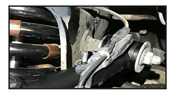
23. Locate the OE ABS wire bracket that was removed from the steering knuckle in Step #6. Using a flat screwdriver, carefully pry open the bracket and remove it from the ABS wire. **Take extra care to not damage the wire.**
