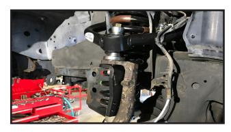
18. Now locate the  $5/16^{\circ} \times 1 1/4^{\circ} \times 2^{\circ}$  round u-bolts, and  $5/16^{\circ}$  flange nuts. Install the u-bolts around the neck of the steering knuckle and through the support bracket mounting holes. Do not tighten the  $5/16^{\circ}$  flange nuts yet.
