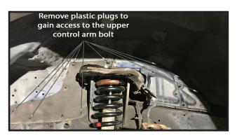
the inner fender that could obstruct the bolt from being bolt to 95 ft lbs. completely removed, if you run into this, you will need to unbolt the wire harness bracket temporarily to gain room to remove the bolt.
