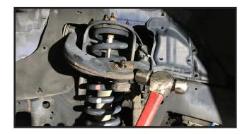
Locate and remove the bracket holding the ABS wire to the very top of the steering knuckle
