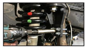
22. Re-install the ABS wire harnes bracket over the welded on bolt on the new upper control arms. Secure using the new 1/4" nut, and 1/4" flat washers from hardware bag 50965NB.
