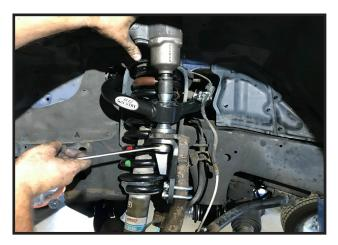
20. Now you can tighten the 5/16" flange nuts so that it closes the gap between the knuckle support bracket and the neck of the steering knuckle.
