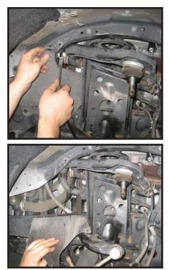
4. Using a pair of large channel locks or similar type tool, Bend the pinch welded lip of the inner fender just enough that the upper control arm bolt will be able to be completely removed. Remove bolt and save. Repeat on passenger side.
