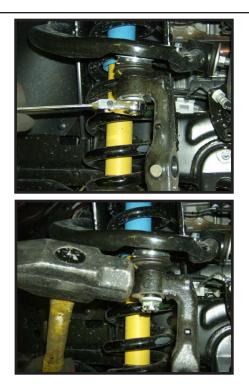
3. Working on the driver side, Remove plastic clips holding rubber spray gaurds to the inner fender. Only remove enough to get to the upper control arm bolt. Repeat on Passenger side.
