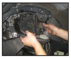
6. Locate the new upper control arms. Locate (8) poly bushings and (4) S10248 sleeves from hardware bag 50930PL, Install the new bushings and sleeves into the new upper control arms. **Special note: Make sure to use** a fair amount of lithium or moly base grease before installing the new bushings and sleeves into the control arms. This will increase the life of the bushing as well as help prevent squeaking.
