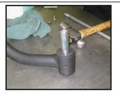
7. Locate the new sert fittings from hardware bag 50930PL. Install the new sert fittings into the new upper control arms. Special note: Make sure not to over tighten and also make sure that the sert fitting is facing towards the outside of the vehicle. This will make for easier access when using a grease gun.
