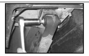
37. Locate the new rear springs. Remove the bushings and sleeves from the new springs and add some lithium or moly base grease to the bushings and sleeves and re-install them back into the new springs. This will help prevent squeaking, the life of the bushings and will also improve ride quality.
