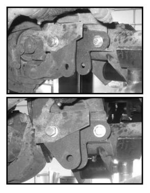
20. Working on the driver side, secure the new brake line relocation bracket to the OE location using the OE hardware. Make sure to use loctite and hand tighten with a wrench. Move back to the 5/16" hardware and add some loctite and torque to **18 ft lbs.** Repeat procedure on the passenger side.
