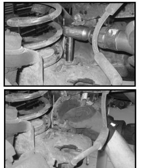
8. Carefully lower down on both hydraulic floor jacks at the same time allowing enough room for the OE coil springs to be removed. Remove the OE coil spring and discard. Repeat
