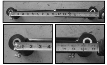
12. Working on the driver side, install the new EZ Flex lower control arm into the OE location using the OE hardware. **Special note: Make sure that when installing the new lower control arms the sert fitting are facing the upward position. Do not tighten at this point.** The lower control arm hardware will be torqued once the weight of the vehicle is on the ground. Repeat procedure on the passenger side.
