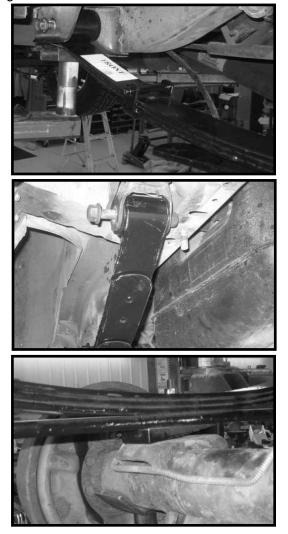
39. Locate the proper u-bolts. Also, locate (8) 1/2" u-bolt washers and (8) 1/2" high nuts from hardware bag 12NW. Working on the driver side, install the u-bolts into the OE location and secure using the new hardware. Torque to **85 ft lbs.** Repeat procedure on the passenger side.
