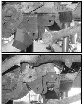
14. Locate (1) S10048 sleeve from hardware bag 43801NB1. Secure the new track bar relocation bracket to the OE pocket using the OE hardware and new sleeve. **Do not tighten at this point.**
