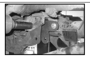
18. Locate (1) 10 mm x 70 mm bolt, (2) 5/16 USS flat washers and (1) 10 mm unitorque nut from hardware bag 43800NB. Install the track bar to the newly installed bracket and secure using the new 10 mm x 70 mm bolt and hardware. Make sure to use loctite and torque to **28 ft lbs.** Special note: If you are not able to install the track bar to the newly installed bracket, this step will need to be performed once the weight of the vehicle is on the ground.
