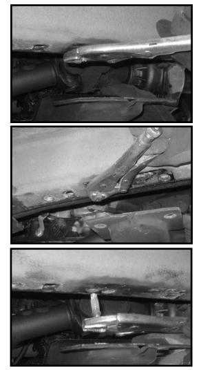
29. Locate the new transfer case cross member. Locate (4) 10 mm x 50 mm bolts, (4) 3/8" lock washers and (4) 3/8" SAE washers from hardware bag 43800NB. Working on the driver side, install the new transfer case spacers between the cross member and the frame. Secure using the new hardware. **Do not tighten at this point.** Repeat procedure on the passenger side.
