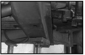
25. Working on the driver side, remove the hardware that attaches the transfer case cross member to the frame. The hardware may be discarded. Repeat procedure on the passenger side.
