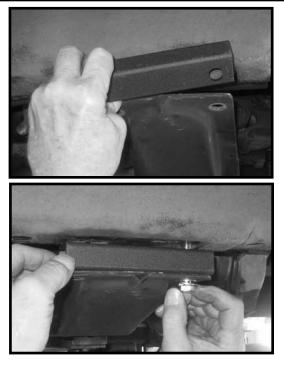
30. Working on the driver side, add some loctite to the newly OE location. The u-bolts and hardware may be discarded. installed transfer case spacer hardware and torque to **28 ft** The upper u-bolt plate can rest on top of the spring. Repeat lbs. Repeat procedure on the passenger side. Carefully remove the hydraulic floor jack from under the transfer case cross member.
