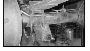
35. Remove the rear brake line from the OE brake line bracket.
