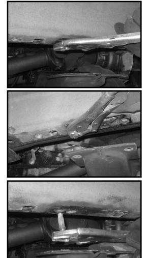
30. Locate the new transfer case cross member. Locate (4) 10 mm x 50 mm bolts, (4) 3/8"lock washers and (4) 3/8" SAE washers from hardware bag 43800NB. Working on the driver side, install the new transfer case spacers between the cross member and the frame. Secure using the new hardware. Do not tighten at this point. Repeat procedure on the
