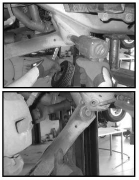
Working on the driver side, remove the coil spring clip from the axle. Save the clip and hardware. Repeat procedure on the passenger side.
