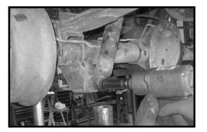
37. Working on the driver side, remove the spring from the OE location. Save the hardware. The spring may be discarded. Repeat procedure on the passenger side.
