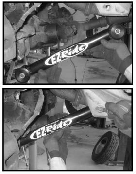
14. Locate the new track bar relocation bracket. Install the new bracket into the OE track bar pocket.
