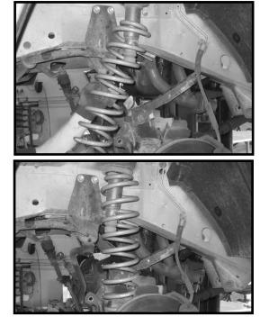
10. Carefully raise up on both hydraulic floor jacks until the newly installed coil springs seat properly into the lower coil spring pockets. Locate and install the OE coil spring clip using the OE hardware on the driver side. Make sure to use loctite and torque to **12 ft lbs.** Repeat procedure on the passenger side.
