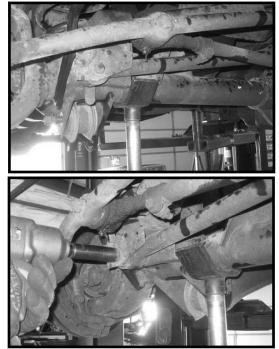
6. Working on the driver side, remove the lower control arm from the frame and axle mount. Save the hardware. The control arm may be discarded. Repeat procedure on the passenger side.
