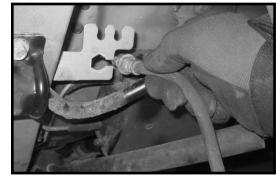
38. Locate the new rear springs. Remove the bushings and sleeves from the new springs and add some lithium or moly base grease to the bushings and sleeves and re-install them back into the new springs. This will help prevent squeaking the life of the bushings and will also improve ride quality.
