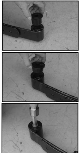
39. Working on the driver side, install the new rear spring
