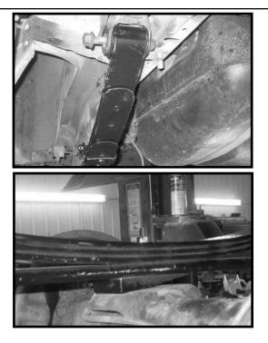
40. Locate the proper u-bolts. Also, locate (8) 1/2" u-bolt washers and (8) 1/2" high nuts from hardware bag 12NW. Working on the driver side, install the u-bolts into the OE location and secure using the new hardware. Torque to 85 ft Ibs. Repeat procedure on the passenger side.
