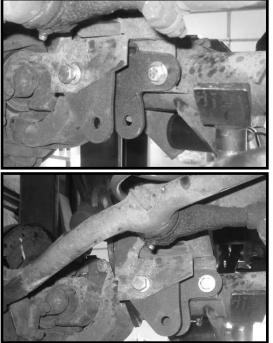
20. Locate (2) BLR05's from hardware bag 43800NB1. Also, locate (2) 5/16" x 1" bolts, (4) 1/4" USS flat washers and (2) 5/16" unitorque nuts from hardware bag 43800NB. Working on the driver side, install the new brake line bracket to the OE brake line bracket and secure using new 5/16" hardware. **Do not tighten at this point.** Repeat procedure on the passenger side.
