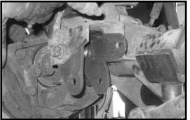
15. Make sure that newly installed track bar bracket is seating flush in the OE pocket. Using the new bracket as a guide, 18. Locate (1) 10 mm x 70 mm bolt, (2) 5/16 USS flat washcarefully drill a 3/8" hole into the OE bracket. ers and (1) 10 mm unitorgue nut from hardware bag
