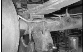
34. Remove the rear brake line from the OE brake line bracket.
