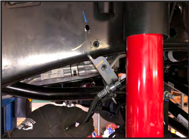
5. Working on both sides, remove the lower mounting hardware for the swaybar endlinks. Save the hardware.
