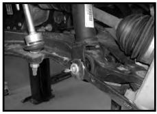
10. Locate (1) new strut spacer and the stock hardware that connected the stock strut into the stock location. Install the new spacer on top of the stock strut and secure using the stock hardware. Make sure to use thread locker or lock tite and torque to 45 ft lbs.
