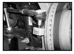
5. Working on the driver side, remove the stock hardware that connects the upper control arm to the knuckle. save the stock hardware.
