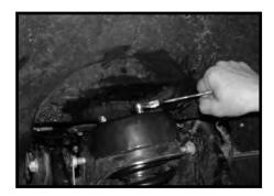
to stock sway bar to the stock end link. Add some thread Tuff Country EZ-Ride Suspension recommends taking locker or lock tite and torque to 32 ft lbs.
