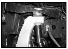
Working on the driver side, remove the upper control arm from the knuckle. Let the knuckle hang. Special note: make sure not to over extended any brake hose and or wires.
