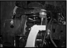
7. Working on the driver side, remove the stock ABS line the stock hardware. Do not tighten at this point. from the stock clip on the backside of the stock knuckle.
