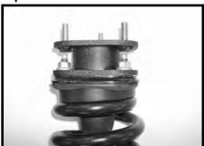
11. Locate (3) 3/8" nylon lock nuts and (3) 5/16" USS flat washers from hardware bag D2P-NB. Working on the driver side, install the newly modified stock strut into the stock upper location. Do not tighten at this point. Secure the lower portion of the strut to the stock lower control arm using
