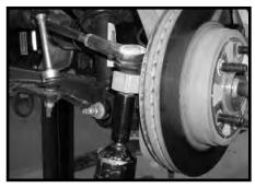
4. Working on the driver side, remove the stock outer tie rod from the the stock knuckle.
