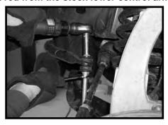
3. Working on the driver side, remove the stock outer tie rod nut that connects the tie rod to the knuckle. Save the stock hardware.
