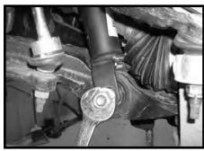
15. Working on the driver side new upper strut hardware add some thread locker or lock tite and torque all (3) nuts to 45 ft lbs.
