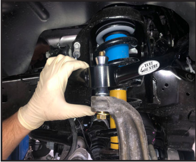
11. Working on the driver side, locate and remove the sway bar end link from the lower control arm. Save the hardware
