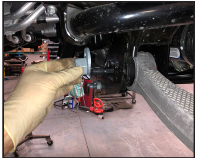
14. Remove both lower control arm cam adjustment bolts and save for later re-installation.
