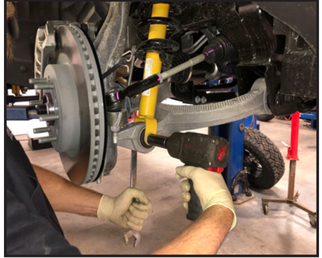
14. Remove both lower control arm cam adjustment bolts and save for later re-installation.
