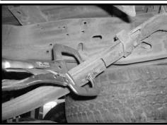
8. Carefully remove the stock centering bolt from the stock location and discard. Special note: Once the stock centering bolt has been removed, the stock over load will fall out. Save the stock over load. Repeat procedure on
