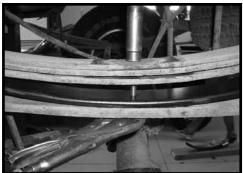
Working on the driver side and using a die grinder, carefully cut off the excess thread from the new centering bolt. Make sure to use thread locker or loctite and torque both the Repeat procedure on the passenger side.
