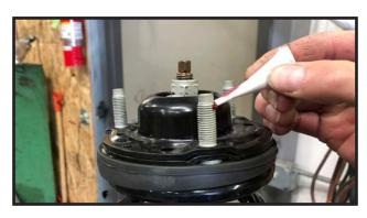
11. Locate Stud extenders in the hardware bag. Install them onto the top hat studs and tighten.
