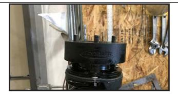
12. Locate the 6 nuts and washers from the hardware bag. Re install driver and passenger side struts into top strut mounts, Using the washers and nuts. Do not tighten.
