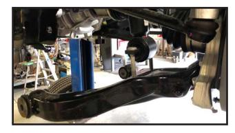
Working on the top strut mounts. Remove the three nuts that holds the srut, and remove the strut. Carful the strut will fall if its not held when last nut is removed. Repeat on passenger side.
