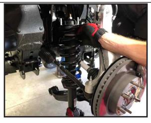
Using vice grip pliers, Remove the dowel pin from the strut top hat on both struts.
