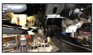
15. Tighten the lower strut studs tell there pulled in all the way in flush. Back nut off one turn, Then Tighten to 90f t lbs.
