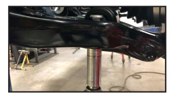
16. Working on the top strut mounts. Tighten the three nuts to 30 ft-lbs
