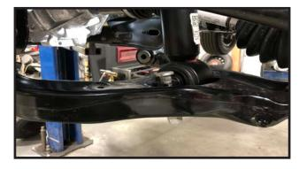
14. Locate OEM lower control arm cam bolt hardware. Using Carefully lower the vehicle back down to the ground and a jack, Raise lower control arms into frame mounts. Install remove the jacks. front and rear cam bolts and nuts into lower control arm mounts. Leave loose.
