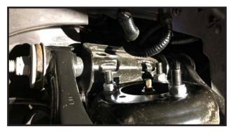
13. On driver and passenger, Raise the lower control arm up to the lower strut mount. Locate the OME lower studs and nuts. Install them into the strut and lower control arm. Leave loose
