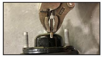
Using a hammer and a vice. Remove the two studs on the lower strut mount. Thread the nut on the stud to prevent damage to the stud. Save Hardware.
