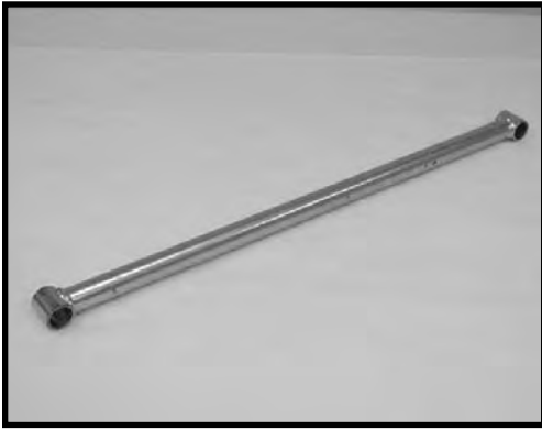
16985-12 (2) Lateral compression struts
