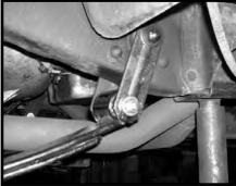
11. Carefully raise up on both hydraulic floor jacks at the same time until they come into contact with the new front springs. Special note: Make sure that the centering bolt
