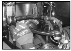
12. Working on the passenger side of the front differential, locate the wiring harness that connects the 4WD control panel to the front differential. Disconnect the 4WD wiring harness from the front differential. Tie the 4WD wiring harness up and out of the way. Special note: Take special care not to kink the wiring.
