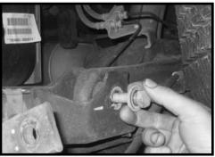
55. Carefully lower down both hydraulic floor jacks at the same time approximately 3". Special note: Take special care not to over extend any brake lines and/or hoses. Working on the driver side, remove the coil spring and set aside. Repeat procedure on the passenger side.
