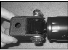
59. Working on the driver side, install the modified shock into the upper and lower location using the OE hardware. Make sure to use loctite and torque to 85 ft lbs. Move back to the new 9/16" hardware and add some loctite and torque to 85 ft lbs. Repeat procedure on the passenger side.
