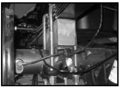
(2) 9/16" x 3" bolt, (4) 1/2" USS flat washers and (2) 9/16" the rear differential. unitorque nuts from hardware bag 14056NB3. Install the point.
