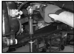
line and set aside. Repeat procedure on the passenger side. 6. Working on the driver side, remove the outer tie rod from the OE knuckle. Save the hardware. Special note: Using a hammer and striking the knuckle will help break the tapper. Take special care not to damage the outer tie rod dust boot during removal. Repeat procedure on the passenger side.
