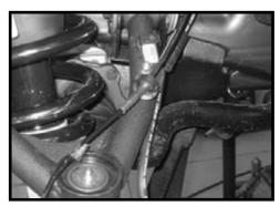
41. Working on the driver side, install the outer tie rod to the OE knuckle using the OE hardware. Make sure to use loctite and torque to 95 ft lbs. Repeat procedure on the passenger
