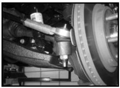
42. Working on the driver side, install the OE end link to the sway bar and lower control arm. Make sure to use loctite and hand tighten
