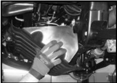
3. Working on the driver side, remove the ABS line from the bracket on the top of the upper control arm pocket. Now disconnect the ABS lines from each other at the quick disconnect. Special note: Take special care not to damage ABS
