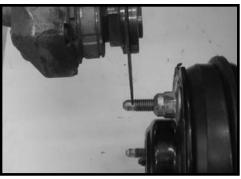
35. Locate the new upper strut spacers. Install the new spacers to the OE struts and secure using the OE hardware. Make sure to use loctite.
