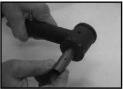
32. Locate (4) SERT04 from hardware bag 14056NB1. have been cut off, remove the OE nuts from each stud. Install the new sert fittings to the new upper control arm. Special note: Take special care not to cross thread during installation and make sure not to over tighten. Hand tighten with an end wrench. Also, make sure that once installed the sert fitting is facing the outside of the vehicle so it will be easy to access with a grease gun.
