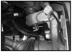
39. Working on the driver side, re-install the CV axle to the front differential using the OE hardware. Make sure to use
