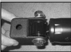
59. Working on the driver side, install the modified shock into the upper and lower location using the OE hardware. Make Tuff Country EZ-Ride Suspension packages (2) sets of sure to use loctite and torque to **85 ft lbs.** Move back to the **instruction sheets with this box kit. (1) is for the installer** new 9/16" hardware and add some loctite and torque to 85 and (1) is for the customer. The (1) for the customer has ft lbs. Repeat procedure on the passenger side.
