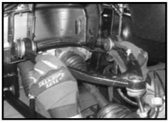
12. Working on the passenger side of the front differential, locate the wiring harness that connects the 4WD control panel to the front differential. Disconnect the 4WD wiring harness from the front differential. Tie the 4WD wiring harcare not to kink the wiring.
