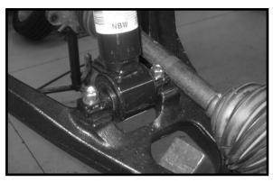
28. Remove the cotter pins and castle nuts from the newly installed control arms. Working on the driver side, install the newly installed upper control arm to the OE knuckle and secure using the new castle nut. Make sure to use loctite and torque to 40 ft lbs. Now install the new cotter pin. Special note: Using a pry bar to gain leverage will help 29. Locate (2) 6 mm flat washers and (2) 6 mm unitorque nuts **be installed.** Repeat procedure on the passenger side.
