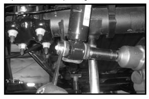
42. Working on the driver side, remove the u-bolts from the OE location and discard the u-bolts and hardware. Set the upper and lower u-bolt plates aside for later re-installation. Repeat procedure on passenger side.
