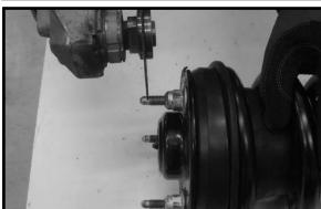
25. Locate the new upper strut spacers. Install the new spacers to the OE struts and secure using the OE hardware.
