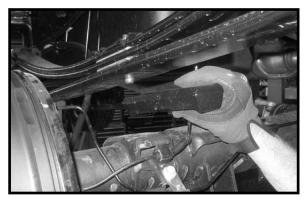
44. Locate (2) new 3" lifted blocks. Working on the driver 47. Locate the new rear shock relocation brackets. Locate side, install the new 3" lifted block into the stock location. (2) 9/16" x 3" bolt, (4) 1/2" USS flat washers and (2) 9/16" Repeat procedure on the passenger side.
