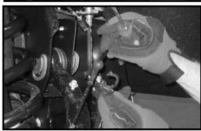
14. Working on the driver side, remove the sway bar end link from the sway bar and lower control arm. Save the end link 16. Working on the driver side, remove the lower hardware and hardware. Repeat procedure on the passenger side.
