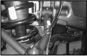
30. Working on the driver side, install the outer tie rod to the OE knuckle using the OE hardware. Make sure to use loctite and torque to 95 ft lbs. Repeat procedure on the passenger side.
