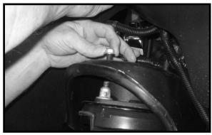
27. Locate (4) 10 mm x 55 mm bolts, (4) 10 mm unitorque nuts and (8) 10 mm flat washers from hardware bag 14059NB. Working on the driver side, secure the lower portion of the OE strut to the lower control arm using the new hardware. Make sure to use loctite and torque to 45 ft lbs. Repeat procedure on the passenger side.
