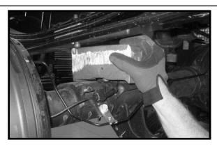
45. Carefully raise up on both hydraulic floor jacks at the same time until the spring assembly sits flush with the newly installed 3" lifted block.
