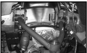
24. Locate the OE struts and upper hardware. Install the OE nuts back to the upper studs of the strut. Using a die grinder, carefully cut off the nipple part of the studs. Special note: Take special care not to cut into the threads. If by chance you do cut into the threads, once you remove the OE nuts the threads will be fixed. Once the nipples have been cut off, remove the OE nuts from each stud.
