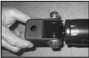
48. Working on the driver side, install the modified shock into the upper and lower location using the OE hardware. Make sure to use loctite and torque to **85 ft lbs.** Move back to the new 9/16" hardware and add some loctite and torque to 85 ft lbs. Repeat procedure on the passenger side.
