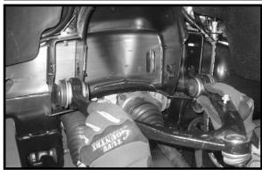
21. Locate the new upper control arms. Locate (8) poly bushings and (4) sleeves from hardware bag 14059PL. Install the new bushings and sleeves into the new upper control arms. Special note: Make sure to use a fair amount of lithium or moly base grease before installing the new bushings and sleeves into the control arms. This will increase the life of the bushing as well as help prevent squeaking.
