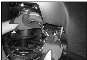
13. Working on the driver side, remove the ABS line from the OE upper control arm. The hardware maybe discarded. Carefully remove the bracket from the ABS line and brake line and set aside. Repeat procedure on the passenger side.
