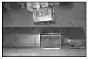
11. Install the newly modified rear cross member back into the OE location using the OE hardware. Make sure to loctite and torque to 45 ft lbs. Special note: Check and double check to make sure that the front differential is not making contact with the modified cross member. If contact occurs, take more material off of the cross member until clearance is achieved.
