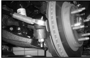
31. Working on the driver side, install the OE end link to the sway bar and lower control arm. Make sure to use loctite and hand tighten.
