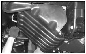
34. Working on the driver side, center and torque the OE Repeat procedure on the passenger side. cam bolts to **95 ft lbs.** Repeat procedure on the passenger side.
