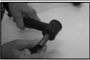
22. Locate (4) SERT04 from hardware bag 14059NB. Install the new sert fittings to the new upper control arm. Special note: Take special care not to cross thread during installation and make sure not to over tighten. Hand tighten with an end wrench. Also, make sure that once installed the sert fitting is facing the outside of the vehicle so it will be easy to access with a grease gun.
