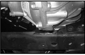
10. Using a die grinder, carefully notch out the OE cross 12. Working on the driver side, remove the ABS line from the bracket on the top of the upper control arm pocket. Now disconnect the ABS lines from each other at the quick disconnect. Special note: Take special care not to damage ABS line during removal. Repeat procedure on the passenger side.
