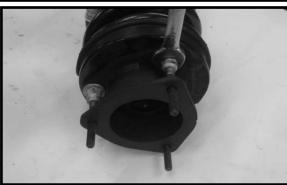
26. Locate (6) 3/8" nylon lock nuts and (6) 5/16" USS flat washers from hardware bag 14059NB. Working on the driv-er side, install the newly modified strut into the upper loca-tion and secure using the new hardware. Make sure to use loctite and torque to **35 ft lbs.** Repeat procedure on the pas-senger side.
