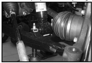
hammer and striking the knuckle will help break the upper strut studs. Remove the nuts holding the strut into the taper. Take special care not to damage the outer tie rod upper location and save. Remove the strut from the vehicle dust boot during removal. Repeat procedure on the pas- and remove and discard the lower attaching clips. Set the strut aside. Repeat procedure on the passenger side.
