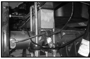
unitorque nuts from hardware bag 14059NB. Install the new shock relocation brackets to the top of the stock shocks and secure using the new hardware. Do not tighten at this point.
