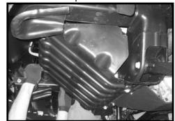
45. Working on the driver side, center and torque the OE cam bolts to **95 ft lbs.** Repeat procedure on the passenger side.
