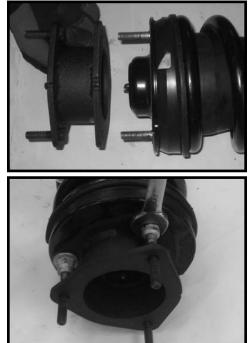
36. Locate (6) 3/8" nylon lock nuts and (6) 5/16" USS flat washers from hardware bag 14056NB2. Working on the driver side, install the newly modified strut into the upper location and secure using the new hardware. Make sure to use loctite and torque to **35 ft lbs.** Repeat procedure on the passenger side.
