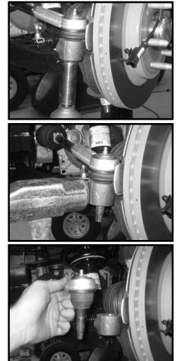
7. Working on the driver side, remove the lower hardware securing the strut to the lower control arm. The hardware may be discarded. Repeat procedure on the passenger side.
