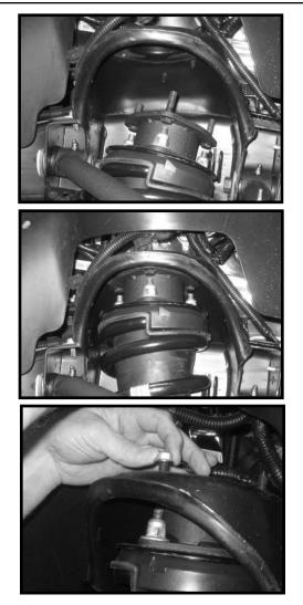
37. Locate (4) 10 mm x 55 mm bolts and (4) 10 mm unitorque nuts from hardware bag 14056NB1. Locate (8) 10 mm flat washers from hardware bag 14056NB2. Working on the driver side, secure the lower portion of the OE strut to the lower control arm using the new hardware. Make sure to use loctite and torque to **45 ft lbs.** Repeat procedure on the passenger side.
