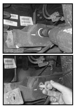
55. Carefully lower down both hydraulic floor jacks at the same time approximately 3". Special note: Take special care not to over extend any brake lines and/or hoses. Working on the driver side, remove the coil spring and set aside. Repeat procedure on the passenger side.
