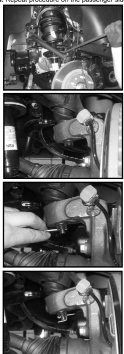
39. Working on the driver side, re-install the CV axle to the front differential using the OE hardware. Make sure to use loctite and torque to **45 ft lbs.** Repeat procedure on the pasar
