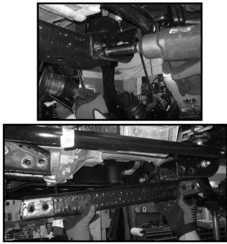
18. With the help from a buddy, carefully remove the front differential from the vehicle and set it on the ground or a work bench.
