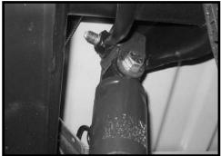
newly installed coil spring and lower lower portion to the 60. Locate the new zip tie in hardware bag 14058NB1. axle. Carefully raise up on the hydraulic floor jack until the Working on the driver side, zip tie the ABS line to the OE coil springs seats properly into the vehicle. Repeat proce-bump stop bracket. Repeat procedure on the passenger side. dure on the passenger side.
