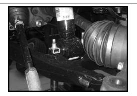
8. Working on the driver side, remove the upper clips off the upper strut studs. Remove the nuts holding the strut into the upper location and save. Remove the strut from the vehicle and remove and discard the lower attaching clips. Set the strut aside. Repeat procedure on the passenger side.
