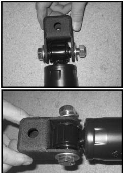
59. Working on the driver side, install the modified shock into the upper and lower location using the OE hardware. Make sure to use loctite and torgue to 85 ft lbs. Move back to the new 9/16" hardware and add some loctite and torgue to 85 ft Ibs. Repeat procedure on the passenger side.
