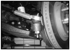
42. Working on the driver side, install the OE end link to the sway bar and lower control arm. Make sure to use loctite and hand tighten.
