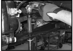
6. Working on the driver side, remove the outer tie rod from the OE knuckle. Save the hardware. **Special note: Using a hammer and striking the knuckle will help break the tapper. Take special care not to damage the outer tie rod dust boot during removal.** Repeat procedure on the passenger side.
