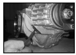
20. Using a die grinder, carefully cut off the shaded area.
