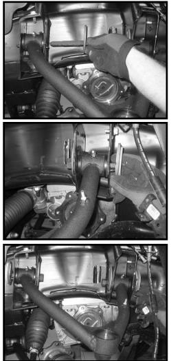
34. Locate the OE struts and upper hardware. Install the OE nuts back to the upper studs of the strut. Using a die grinder, carefully cut off the nipple part of the studs. Special note: Take special care not to cut into the threads. If by chance you do cut into the threads, once you remove the OE nuts the threads will be fixed. Once the nipples
