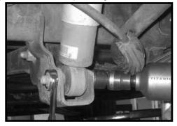
53. Working on the driver side, remove the end link from the OE mount and sway bar. The sway bar and the lower hardware may be discarded. Save the upper hardware. Repeat procedure on the passenger side.
