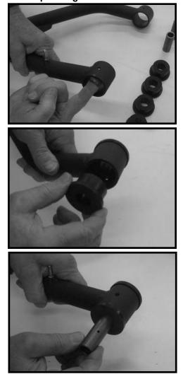
32. Locate (4) SERT04 from hardware bag 14056NB1. have been cut off, remove the OE nuts from each stud. Install the new sert fittings to the new upper control arm. Special note: Take special care not to cross thread during installation and make sure not to over tighten. Hand tighten with an end wrench. Also, make sure that once installed the sert fitting is facing the outside of the vehicle so it will be easy to access with a grease gun.
