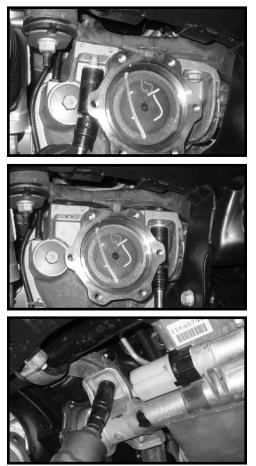
21. Working on the passenger side and using an air chisel, note: If you do not have access to an air chisel, the passenger side OE bracket will need to be removed from the vehicle to have these bolts removed.
