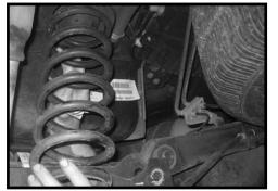
56. Locate the new coil spring spacer and the coil spring washer. Also, locate (2) 3/8" x 3" bolts, (2) 5/16" USS flat washers and (2) 3/8" flange nuts from hardware bag 14058NB1. Working on the driver side, install the coil spring spacer to the upper coil spring pocket using the coil spring washer on the top of the coil spring pocket and secure using the new 3/8" hardware. Make sure to use loctite and torgue to **28 ft lbs.** Repeat procedure on the passenger side.
