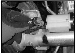
13. Carefully remove the front drive line from the front differential. Save the hardware. Carefully tie the front drive line up and out of the way.
