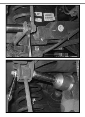
OE track bar mount. Save the hardware for later re-installation.
