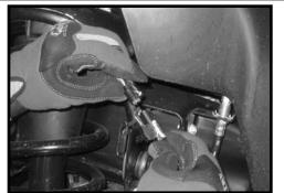
4. Working on the driver side, remove the ABS line from the OE upper control arm. The hardware maybe discarded. Carefully remove the bracket from the ABS line and brake line and set aside. Repeat procedure on the passenger side.
