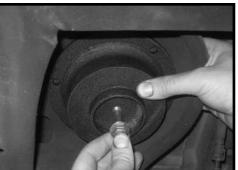
57. Working on the driver side, locate and install the coil spring back into the vehicle. Install the upper portion to the
