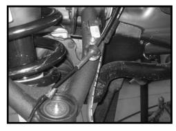
41. Working on the driver side, install the outer tie rod to the OE knuckle using the OE hardware. Make sure to use loctite and torque to **95** ft lbs. Repeat procedure on the passenger side.
