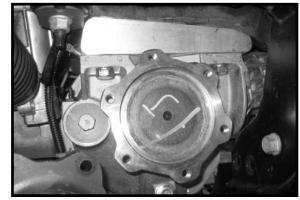
25. Locate (4) 12 mm x 35 mm bolts from hardware bag 14056NB1. Also, locate (2) 12 mm lock washers and (2) 12 mm fender washers from hardware bag 14056NB3. Secure the passenger side of the differential to the newly installed passenger side differential spacer using the new hardware. Make sure to use loctite and torque to **55 ft lbs.**
