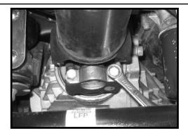
14. Working on the driver side, remove the CV axle from the front differential flange. Save the hardware. Special note: Take special care not to over extend the CV axle during removal. Rest the CV axle on the lower control arm. Repeat procedure on the passenger side.
