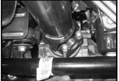
30. Re-install the rear cross member to the driver and passenger side rear lower control arm drop pockets using the OE hardware. Make sure to use loctite and torque to **55 ft Ibs.**
