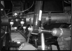
53. Working on the driver side, remove the u-bolts from the 57. Locate (4) 9/16" x 2 9/16" x 11 5/8" square u-bolts. OE location and discard the u-bolts and hardware. Set the Locate (8) 9/16" u-bolt high nuts and (8) u-bolt washers from upper and lower u-bolt plates aside for later re-installation. Repeat procedure on passenger side.
