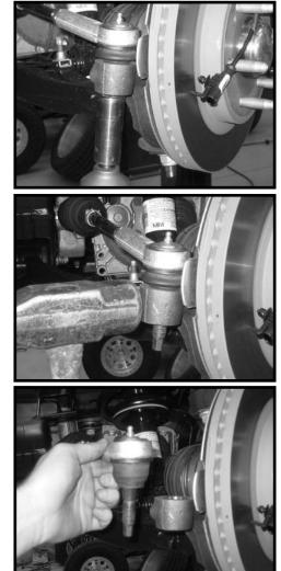
Working on the driver side, remove the lower hardware securing the strut to the lower control arm. The hardware may be discarded. Repeat procedure on the passenger side.
