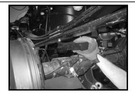
55. Locate (2) new 3" lifted blocks. Working on the driver side, install the new 3" lifted block into the stock location. Repeat procedure on the passenger side.
