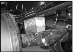
hardware bag 916NW. Also, locate the upper and lower ubolt plates. Working on the driver side, install the new u-bolts into the stock location and secure using the new 9/16" high nuts and washers. Special note: Make sure to re-install the upper and lower u-bolt plates into the stock location. If need be, cut off the excess threads off each leg of the newly installed u-bolts. Torque to 120 ft lbs. Repeat procedure on passenger side.
