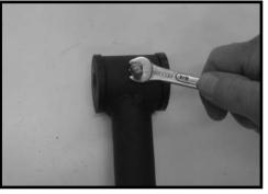
33. Working on the driver side, install the new upper control arm into the OE location using the OE cam bolts. **Do not** tighten at this point. Repeat procedure on the passenger side.
