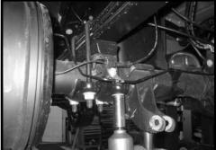
54. Carefully lower down both hydraulic floor jacks at the same time approximately 3". **Special note: Take special care not to over extend any brake lines and/or hoses.** Working on the driver side, remove and discard the stock rear block. Repeat procedure on the passenger side.
