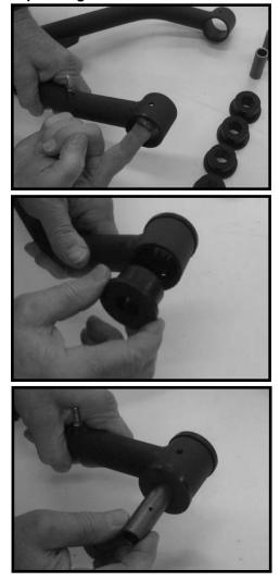
32. Locate (4) SERT04 from hardware bag 14056NB1. have been cut off, remove the OE nuts from each stud. Install the new sert fittings to the new upper control arm. Special note: Take special care not to cross thread during installation and make sure not to over tighten. Hand tighten with an end wrench. Also, make sure that once installed the sert fitting is facing the outside of the vehicle so it will be easy to access with a grease gun.
