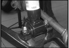
38. Locate (2) cotter pins and (2) castle nuts from hardware Repeat procedure bag 14056PL. Working on the driver side, install the newly on the passenger installed upper control arm to the OE knuckle and secure side.
