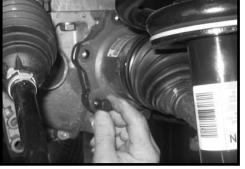
40. Locate (2) 6 mm flat washers and (2) 6 mm unitorque 44. Install the OE skid plate using the OE hardware. Make nuts from hardware bag 14056NB2. Working on the driver sure to use loctite and torque to **40 ft lbs.**
