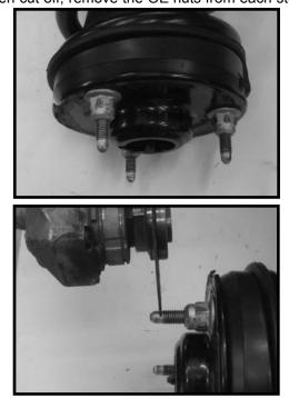
35. Locate the new upper strut spacers. Install the new spacers to the OE struts and secure using the OE hardware. **Make sure to use loctite.**
