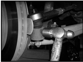
3. Working on the driver side, loosen but do not remove the nut that connects the upper control arm ball joint to the knuckle. Carefully break the taper from the upper control arm ball joint and the knuckle. Once the taper has been broken, remove the nut and set aside. Special note: Take special care not to damage the upper control arm ball joint or the dust boot. A helpful tip is to hit the knuckle with a hammer to break the taper. Repeat procedure on the passenger side.
