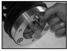
8. Locate the modified driver side strut. Also, locate (3) 7/16" x 1" bolts, (3) 3/8" USS flat washers and (3) 7/16" lock washers from hardware bag 12000NB. Install the modified driver side strut into the **PASSENGER** side upper location and secure using the new 7/16" x 1" bolts and hardware. **Do not tighten at this point.**
