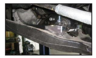
9. Move back to the upper ball joints and tighten. Torque to 37 ft lbs.
