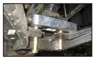
8. Locate (4) 10mm x 1.5 x 80mm bolts if your lower control arm is made of steel, and (4) 10mm x 1.5 x 90mm bolts if your lower control arms are made of aluminum. Also locate (8) 10mm washers and (4) 10mm unitorque nuts. Install the new hardware to secure the lower strut mount with the newly installed 12001-01 spacers. Torque to 35 ft lbs.
