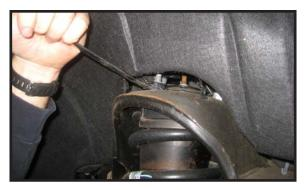
6. Working on the driver side, loosen, but DO NOT remove the upper control arm nut. Using a hammer, carefully hit the steering knuckle to break the ball joint taper free. Repeat on passenger side.
