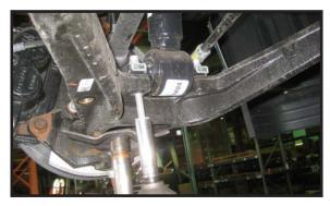
On both sides of the vehicle, remove the nut clips from the lower strut mounts and discard.
