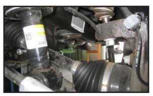
7. You should now have enough space between the lower 12. Re-install tires and wheels. strut mount to install the new 12001-01 spacer. Install on both sides of the vehicle.
