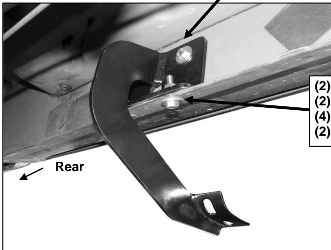
(Fig 3) Driver side-rear Mounting Bracket location
