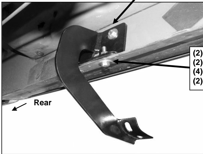
(Fig 3) Driver side-rear Mounting Bracket location
