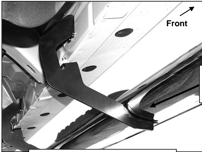
(Fig 8) Driver/left brackets installed
