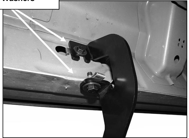
(Fig 7) Example of Bracket bolted to 8mm Clip Nuts on mounting tab and inner body panel
