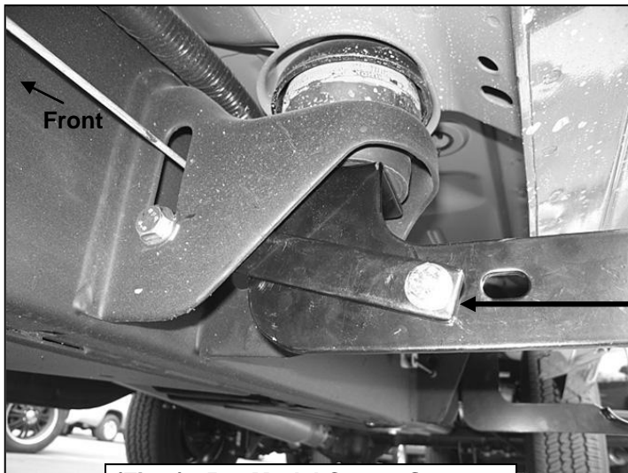
(Fig 6) 1500 Model Center Support Bracket Installation Pictured
