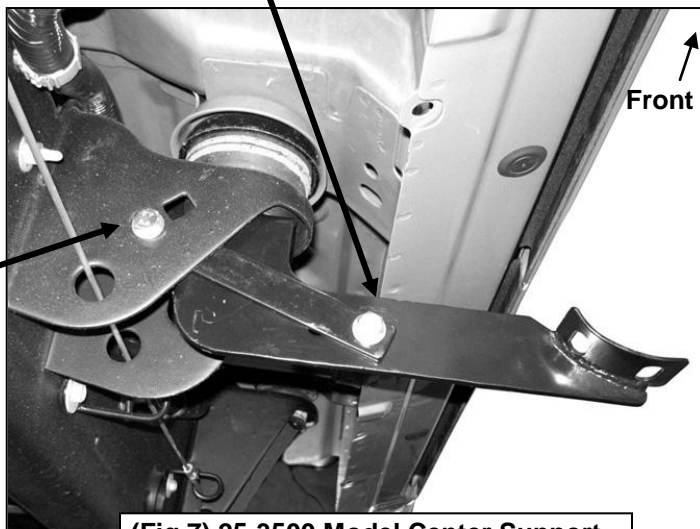
(Fig 7) 25-3500 Model Center Support Bracket Installation Pictured
