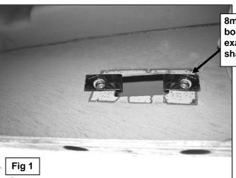
8mm Clip Nuts (hole in body panel shown for example only-location and shape may differ slightly)
