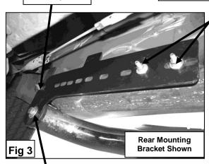
8mm x 30mm Hex Bolts 8mm Lock Washers 8mm Flat Washers 8mm Hex Nuts
