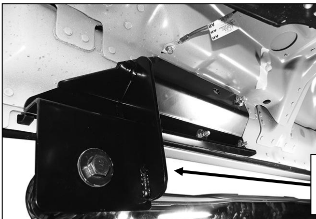
(Fig 5) Passenger side front Bracket installation
