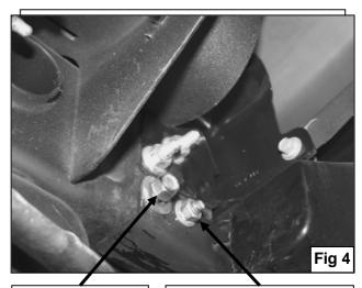
12mm Bolt Plate 12mm Lock Washer 12mm Hex Nut 12mm Flat Washer
