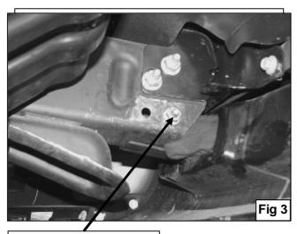
Factory Hardware or 12mm x 140mm Hex Head Bolt 12mm Lock Washer 12mm Hex Nut 12mm Flat Washers
