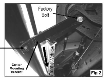
10mm x 25mm Hex Head Bolt 10mm Lock Washer 10mm Flat Washer
