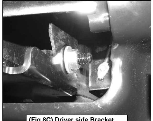
(Fig 8C) Driver side Bracket installation pictured from front
