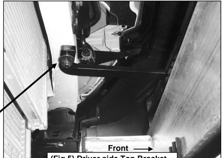
(Fig 5) Driver side Top Bracket installation pictured from below
